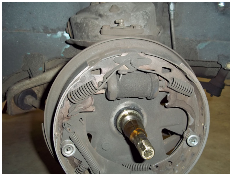
New racing drum setup after one track weekend. Note SS brake line, vented backing plates, 1" bore cylinder and unequal wear on front and rear shoes. Carbon metallic race shoes generate much heat and dust - drums were throw-away items due to extreme "bellling".
